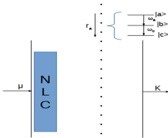
**Figure .1. Schematic representation of a non-degenerate three level laser with a parametric amplifier and a thermal reservoir.**
